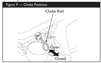
**NOTE:** For a warm engine, be sure the choke is in the OPEN position (no choke).
